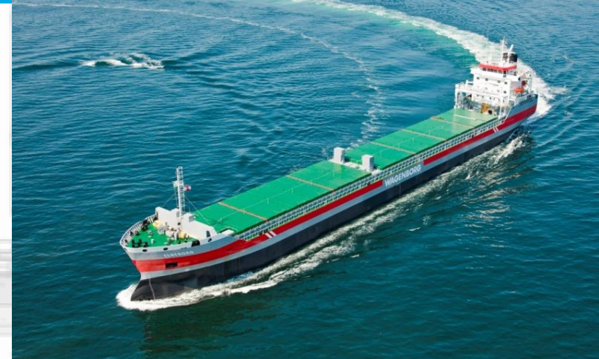
MV Elbeborg of Wagenborg Shipping 12000 DWT General Cargo MPP 4500 kW Wartsila 9L32C
